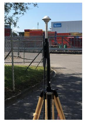
**Figure 1.** Tri-axial Satimo INSITE Free electric-field probe (at a height of 1.5 m) in line-of-sight of a fifth generation new radio base station in Bern, Switzerland.
